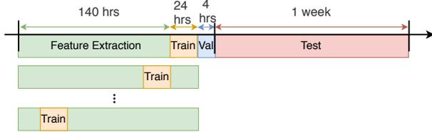
**Figure 1: Data partitioning.** We use a 24 hour sliding window approach to create the training set. To maximize training data all models are validated on a small 4 hour validation set forward in time. Public and private leaderboard test data is taken from the following week.
