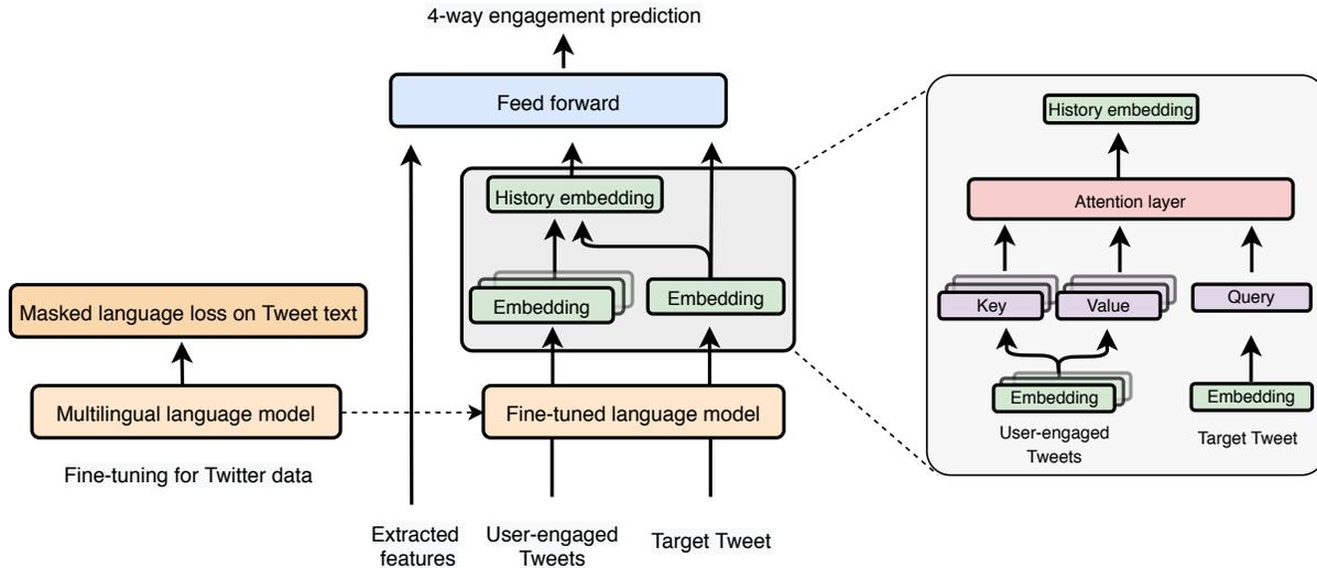
**Figure 2: Model Architecture.** Multilingual language model (M-BERT, XLM-R) is first fine-tuned with Twitter data using unsupervised masked language loss. The fine-tuned model is then used to extract embeddings for target tweet and most recent historical tweets that target user engaged with. Tweet embeddings are aggregated with attention and combined with extracted features in a feed forward network to output 4-way engagement prediction.
